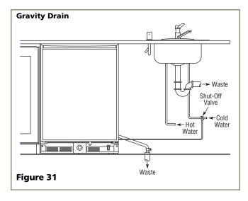
If using a Gravity Drain:
